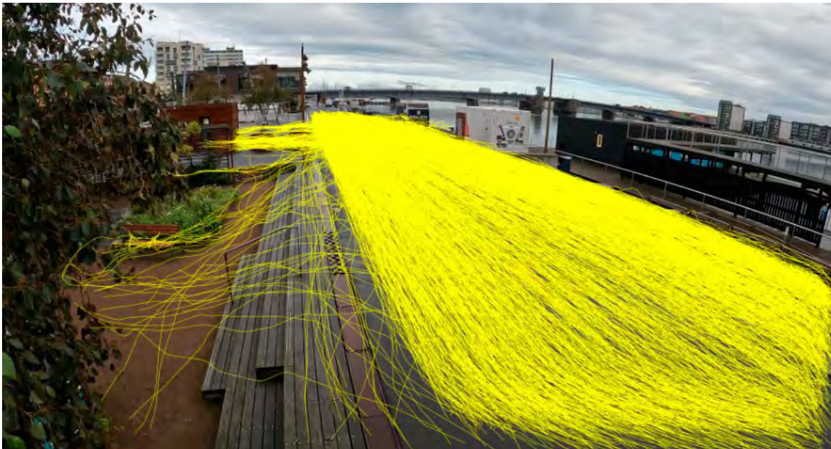
Pedestrians in the area in the period 07:58–16:40 on 28 August tracked with GoodVision. A total of approx. 750 pedestrians in each direction.
