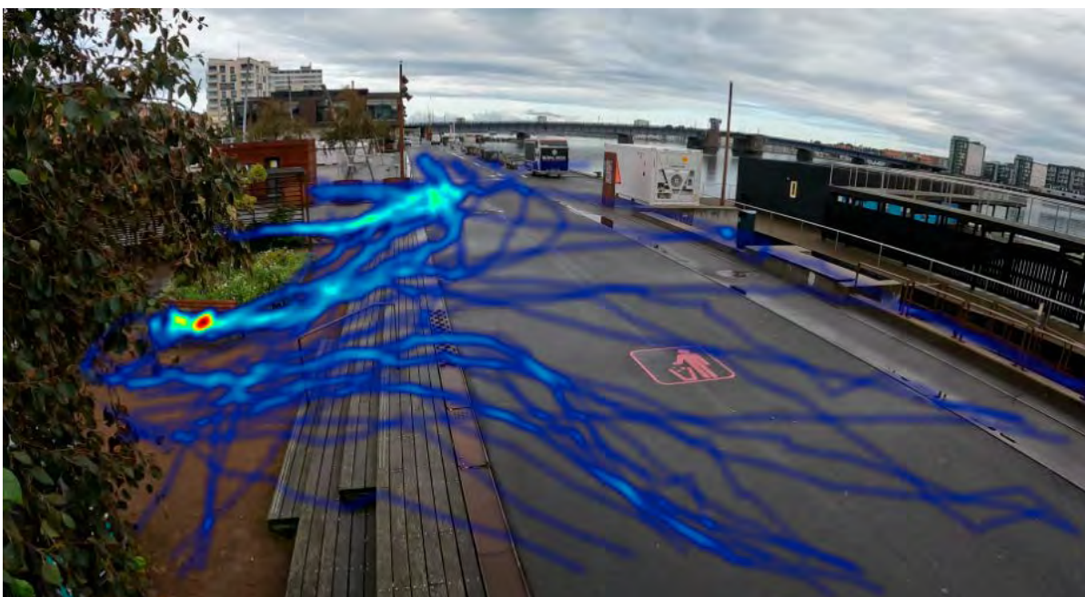
Movement patterns for the people who cross the steps between the promenade and the city garden, established using GoodVision.
