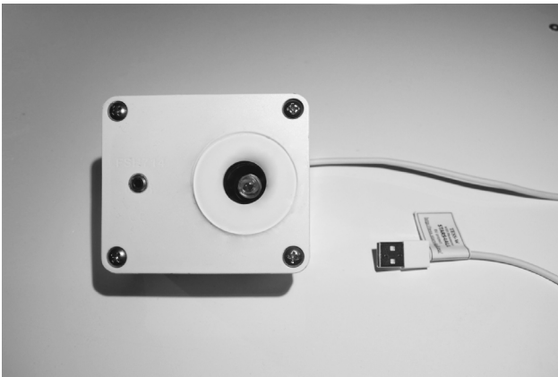
Tess W photometer, a device which can be used to measure night sky illumination. Source: https://tess.stars4all.eu/faqs/ . Photo of the left by Lucía García and photo of the right by Alexis Mancilla
