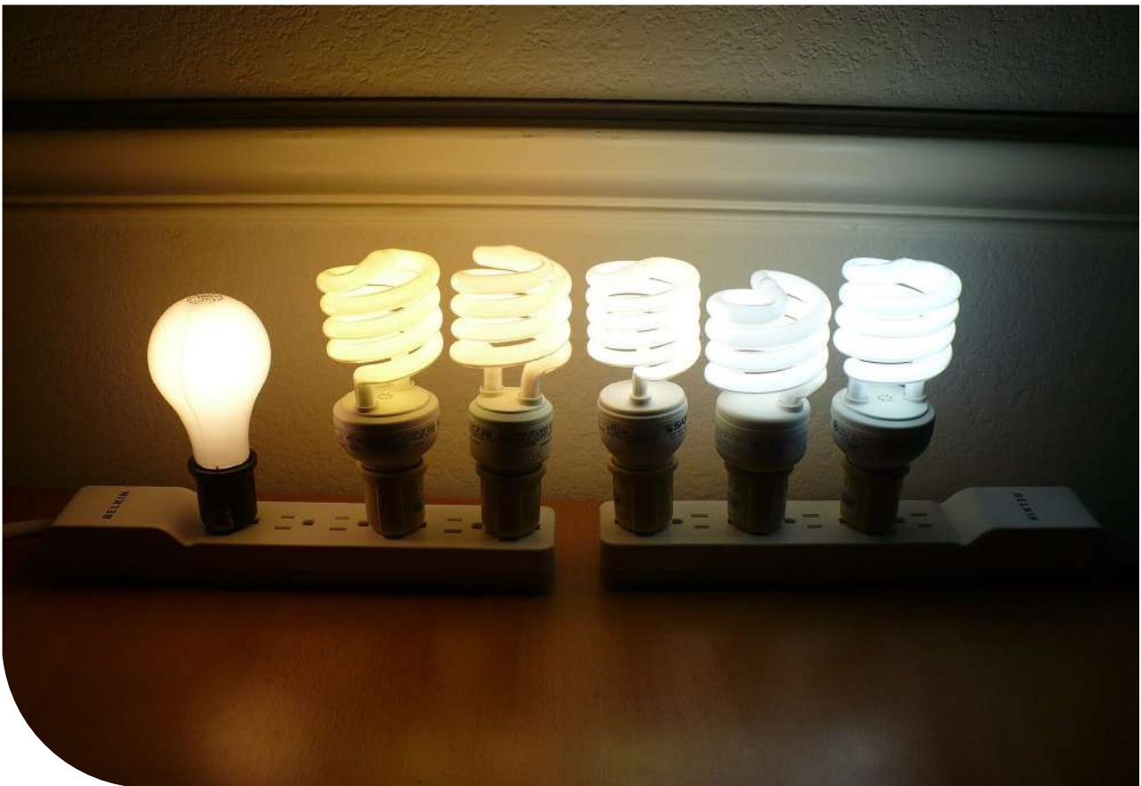
Comparison of correlated colour temperature (CCT) of five lamps (indoor compact fluorescent light bulbs). From left (warmer yellow) to right (cooler blue): 2700K, 3500K, 4100K, 5500K, 6500K CFL. The warmer yellow lower CCT light, is suggested for exterior lighting due to the lower amount of blue light – known to be harmful to many nocturnal species. Source: User: Splarka, Public domain, via Wikimedia Commons, https://commons.wikimedia.org/wiki/File:Color_temperature_comparison_of_5_CFLs.jpg
