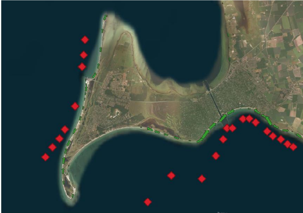
Figure 2. The results for the longshore sediment transport estimates around the Falsterbo peninsula. The green arrows indicate the modeled direction and magnitude of the net transport. The red dots indicate the wave model grid nodes where the wave information was extracted for the longshore sediment transport estimates. The colored background represents the bathymetry scaled from green (shallow) to red (deep).
