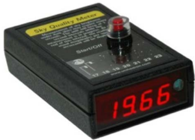
Figure A8.1. Unihedron Sky Quality Meter. Source: IDA
