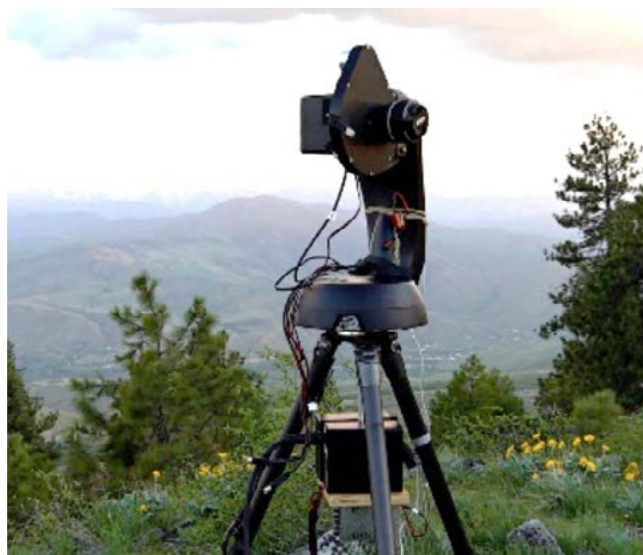
Figure A8.3. NPS All-Sky Camera. Source: NPS
