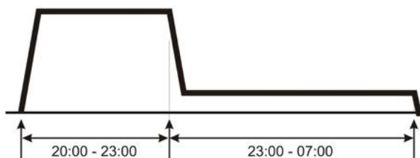
Figure A4.6. Sample illumination schedule for low ecological impact. Actual times will vary depending on time of year, daylight versus standard time, latitude, etc. The graph starts at sunset and ends at sunrise. The raised part indicates desired lighting for evening activity. The lower part to the right represents lights turned off or dimmed during dark time, the rest of the night till sunrise. Source: Robert Dick
