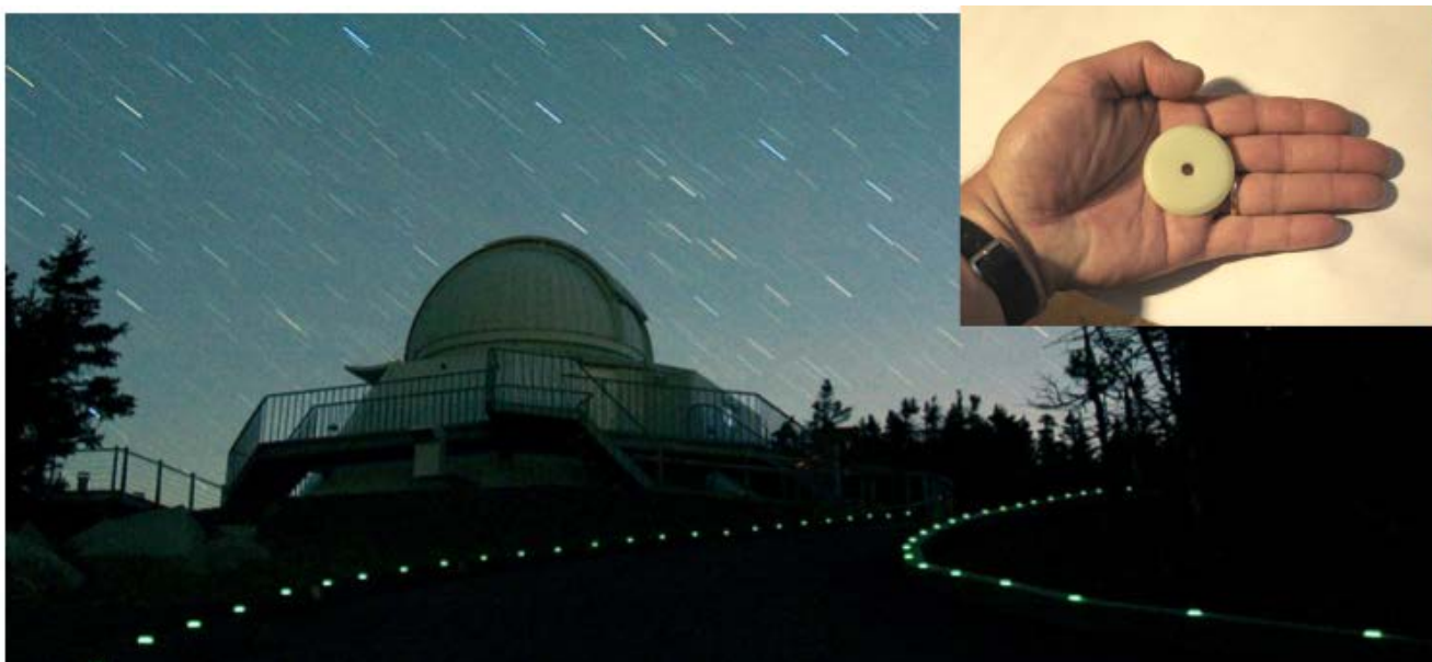
Figure A5.2. Phosphorescent road markers at Mont-Mégantic. Source: Guillaume Poulin
