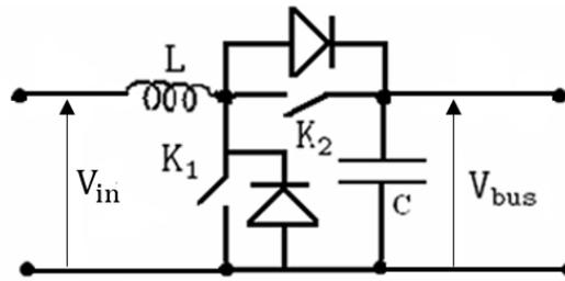
Figure 8: Retained DC-DC bidirectional topology for the BESS side.
