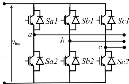
Figure 10: Retained DC-AC topology for the HP side.
