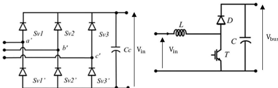
Figure 9: Retained AC-DC followed by DC-DC topologies for the WT side.
