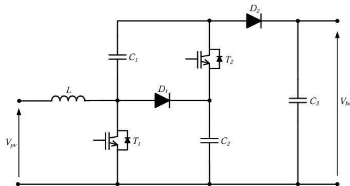
Figure 7: Retained DC-DC topologies for the PV side.
