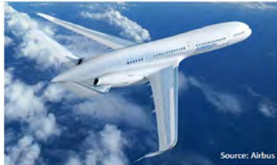
Propulsion integrated in airframe for low noise
