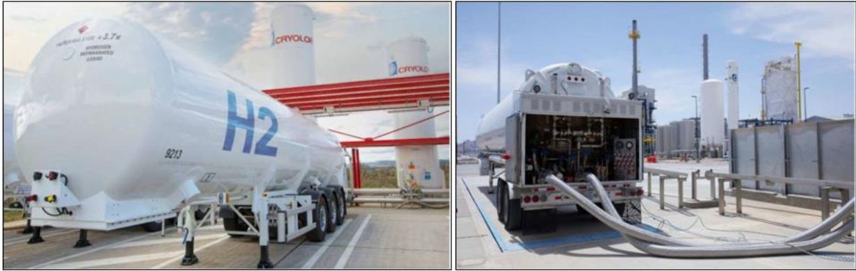
Liquid trailer for transport of 4000 kg under 1 to 4 bar at a cryogenic temperature.
