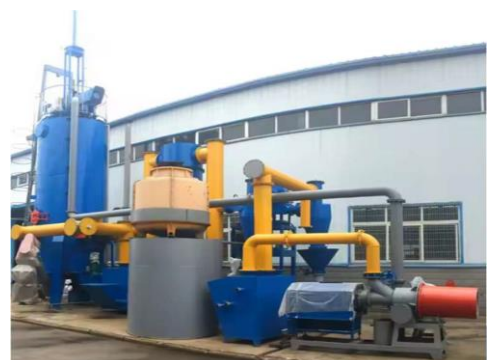
Automatic Industrial Biomass Pyrolysis Gasifier.
