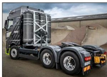
Hydrogen-powered truck from MAN with the arrangement of the tanks.
