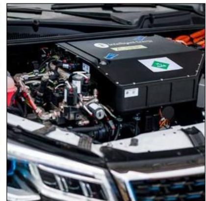
BOP also small and compact? Compact fuel cell systems of a car. The power outputs are 150 kW ratio.
