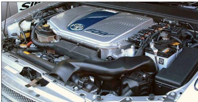
BOP also small and compact? Compact fuel cell systems of a car. The power outputs are 150 kW ratio.
