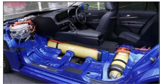
Toyota Mirai with installation of the hydrogen tanks.
