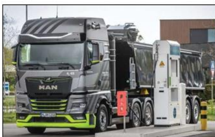
Hydrogen-powered truck from MAN with the arrangement of the tanks.
