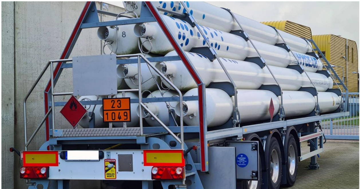
Setup of a tube trailer with the mandatory symbols.
