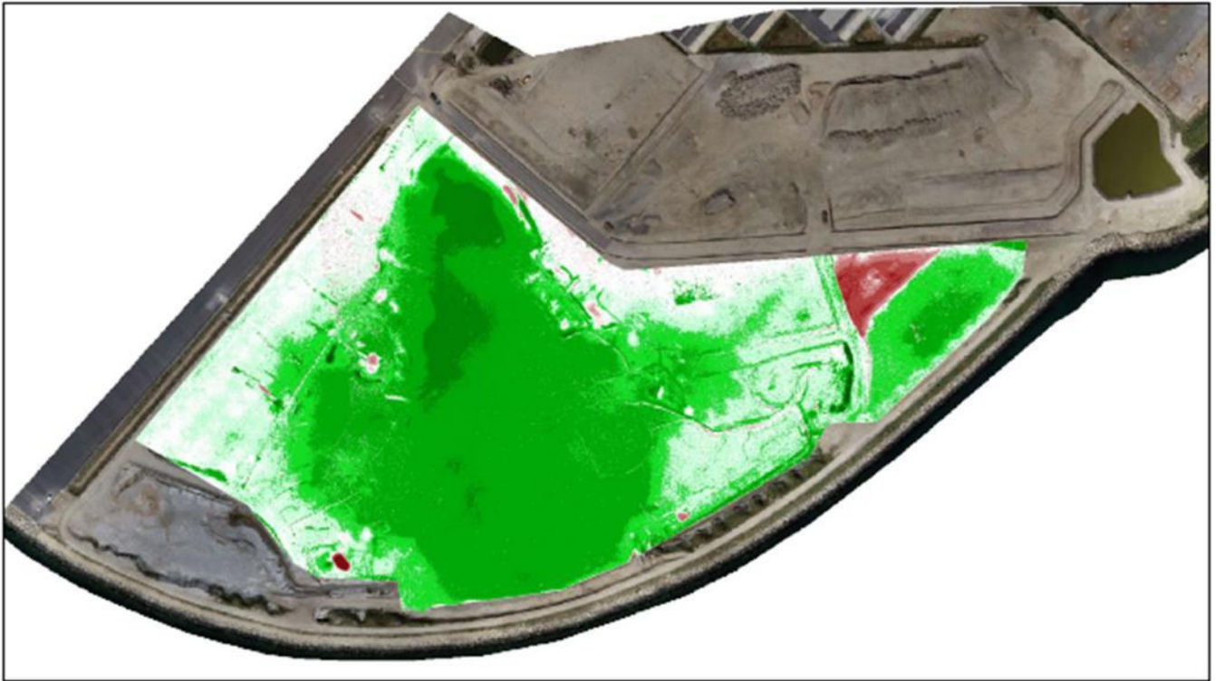
Figure II-3: Topographic survey - Differential DTM between October 2023 and February 2024 - New Polder [21].
