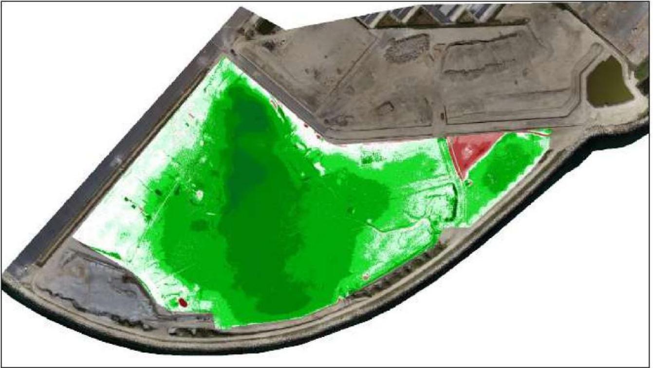
Figure II-5: Topographic survey - Differential DTM between October 2023 and April 2024 - New Polder [21].
