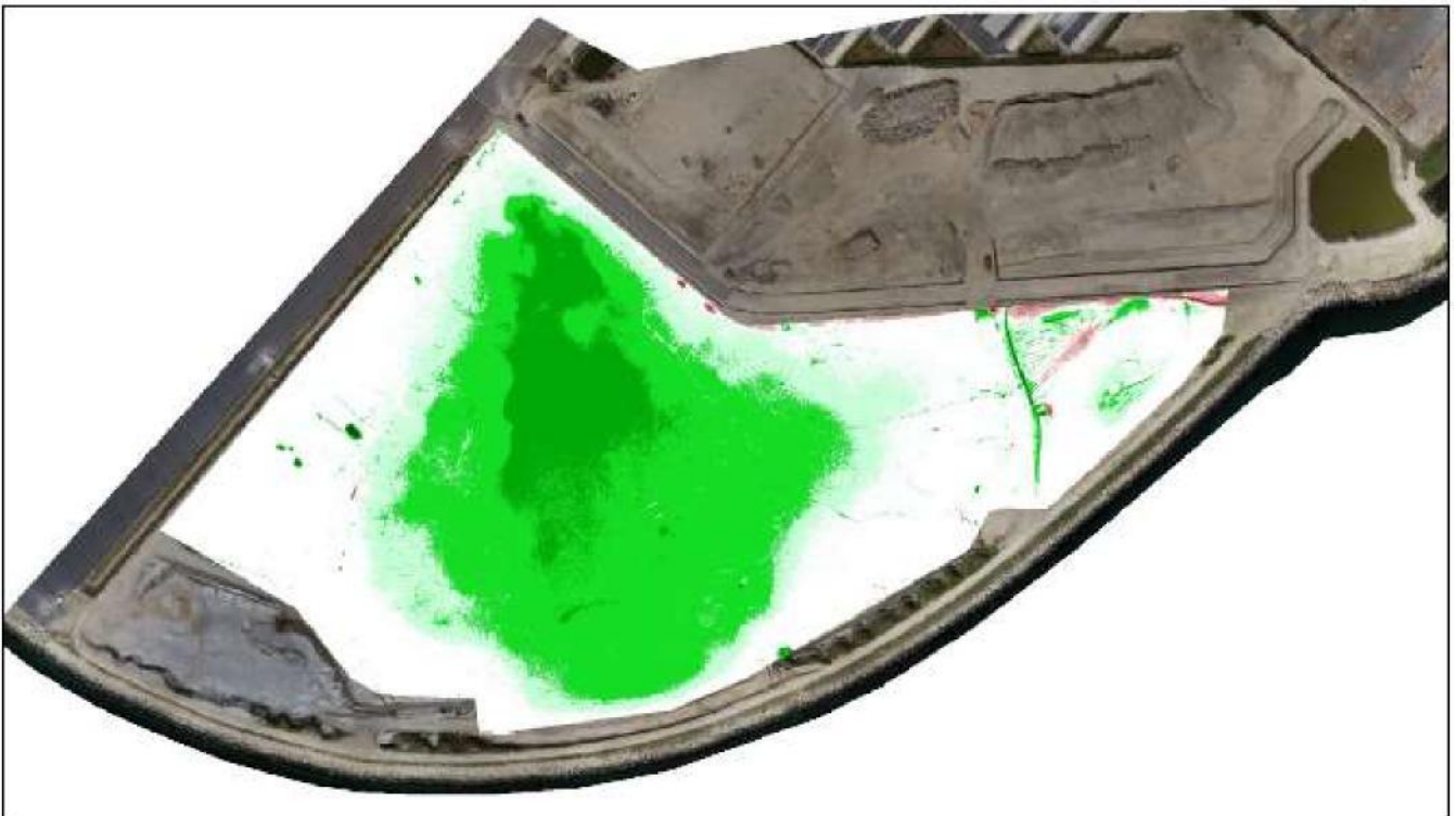
Figure II-4: Topographic survey - Differential DTM between February 2024 and April 2024 - New Polder [21].
