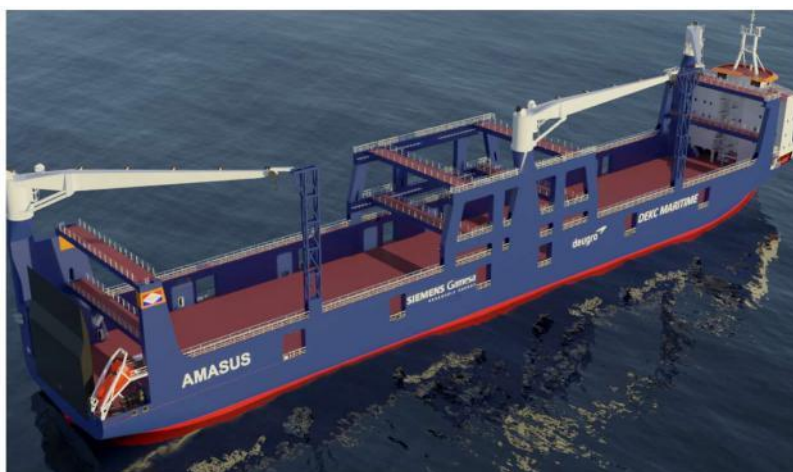
Figure I-10: Rotra Futura, future RORO SGRE transport vessel, 167 x 26 m
