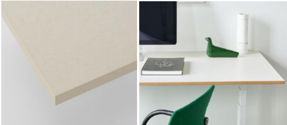
Figure 36: The Kvadrat Really Textile Tabletop™ is a new recycled composite product, made of pre- and post-consumer end-of-use textile (cotton, polyester or wool), pressed with 30% of binder. Textile Tabletop™ is pre-coated, either finished or semi-finished, and is directly applicable to existing and new table frames with no need for additional surface and edge treatment.
