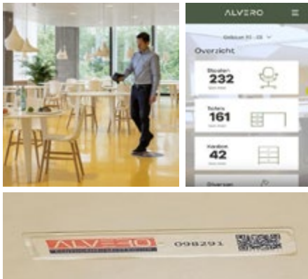
Figure 87: Specialized in the renting of office furniture, Alvero integrates a furniture management platform for its clients. Thanks to a specific reader and an RFID tag affixed on each furniture, the customer is able to scan each furniture item over a distance of 50 meters, and get the inventory per area, room or floor. Information is also communicated like brand and model of furniture, maintenance history and foreseen maintenance cost, depreciation and residual value, circular economy value. This platform was developed by Alvero first for an internal need of inventory management.
