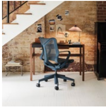
Figure 30: Herman Miller designed office chairs where the usual upholstery PU foam material is removed, and replaced by a polymeric flexible net stretched in a thin but strong flexible frame. Less material for a total support. credit: Photo by Pippa Drummond, courtesy of Herman Miller.
