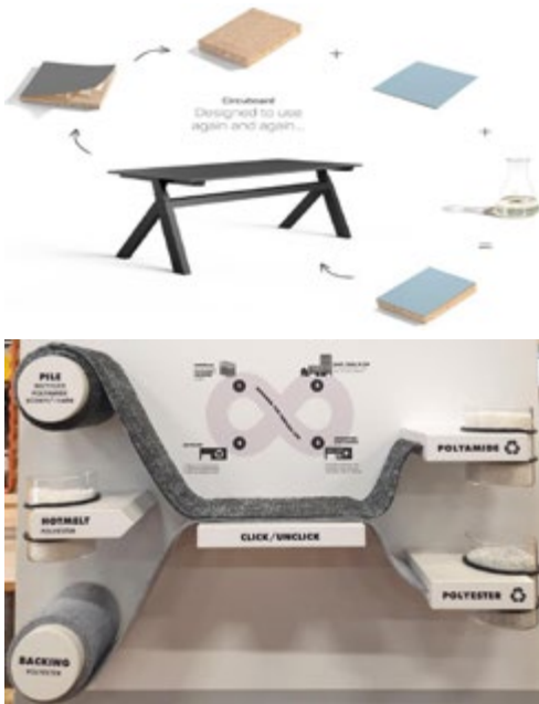
Figure 70: glues are necessary in some cases in furniture, making separation of the materials nearly impossible. The Niaga® tag is a click-unlock polyester adhesive that allows for easy ungluing of the materials by simply heating. This adhesive is used for instance:
