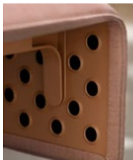
Figure 28: The aluminum structure of the Circulus sofa from OFFECT has a lower thickness and is perforated with holes to reduce the material use. The shape of the flanged holes brings enough stiffness to compensate the material removal.
