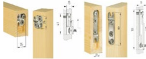
Figure 75: The DUO-System® is a dovetail frame connector (fast assembly without tool, self-tightening). Knapp®
