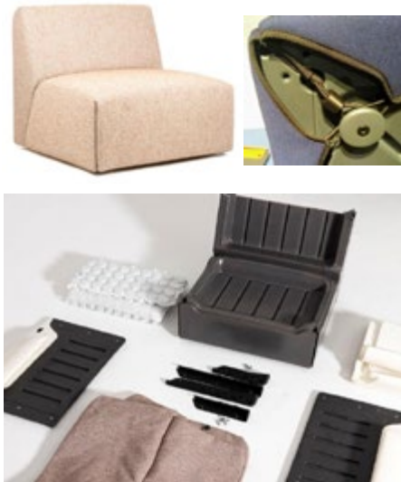
Figure 65: COSTUME is a modular sofa from Magis, where individual components can be easily dismantled and replaced. Thanks to the elastic loops hooked into the base, the sofa can be undressed when needed for washing or replacing the cover. Even the thin polyurethane foam insert can be taken out and cleaned. The disassemblable system makes the components recyclable, and in addition, the polyethylene structure is made of recycled material
