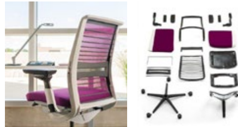
Figure 59: First C2C labelled product, the office chair Think from Steelcase takes approximately five minutes to disassembly and requires only common hand tools. It was designed with fewer parts and with a third of recycled materials.
