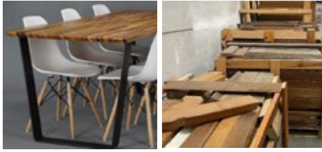
Figure 98: La Ressourcerie Namuroise, a Belgian waste collector and distributor of reused products, has also an upcycling activity to valorize the recovered furniture that are not suitable for selling: they are cut and transformed into glulam (glued laminated timber), suitable for making new furniture like desks, shelves, or interior design. For now, the manufacturing process of glulam is manual, involving high product price. To reduce the production cost and increase the production volume, an industrial production line is put into place at the time of writing this guide.
