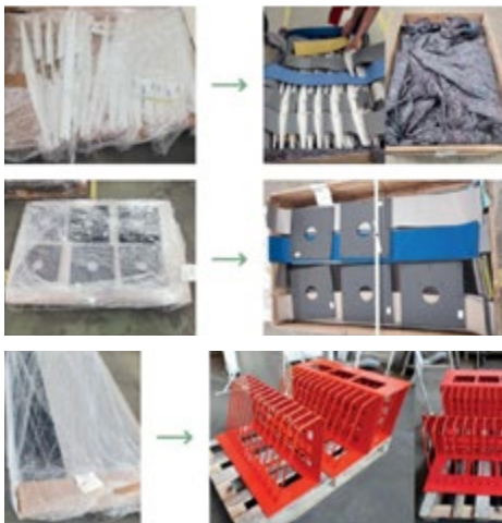
Figure 85: NowyStyl has taken measurements to reduce the single-use cardboard and plastic film: reusable protective cover and blankets that come from their own fabric scraps; tie-down straps and spacers for the internal logistics between the factories. These solutions allow to avoid the use of several tons of plastic films since 2020.
