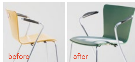
Figure 94: The Fair Furniture Group opened its Circular Center in The Netherlands, a location where all circular operations on second-hand furniture take place, such as refurbishing and repairing. All products are leaving the Circular Center with a Fair Furnished label. This example is the refurbishment of a Vico Duo chair by Fritz Hansen. Main steps involved are: disassembling the shell from the frame, cleaning the metal frame, sanding and repainting the shell with a spray gun, upholstering and inserting it on the shell, reassembling. This refurbishment allows to recover the whole chair's component, and making it more comfortable by adding few upholstery materials (fabric, foam and wooden plate). The painting of the shell is a simple and fast operation to refurbish the shell that shows signs of wear.
