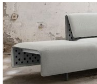
Figure 28: The aluminum structure of the Circulus sofa from OFFECT has a lower thickness and is perforated with holes to reduce the material use. The shape of the flanged holes brings enough stiffness to compensate the material removal.
