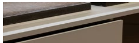
Figure 22: The FENIX laminates are made of several layers of paper impregnated in a thermosetting resin and pressed through heat and pressure to obtain a homogeneous non-porous product. The outer surface is treated with next generation acrylic resin which is hardened and fixed through an electron beam curing process. The result is a surface with properties of thermal healing of superficial micro-scratches: heating the surface can reactivate the cross-linked polymer network that will remove micro-scratches, making a surface highly durable.
