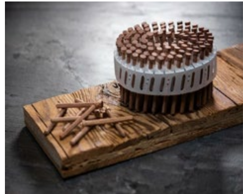
Figure 43: LIGNOLOC® is a patented wooden nail that enables a new fastening technology of wood with wood, replacing the usual steel nails. Applied with a pneumatic nailer, the connection is robust and non-detachable. By avoiding using steel nails in massive wood furniture, not only the recyclability is bettered, but also the reconditioning and remanufacturing of furniture are enhanced – typically, cutting and sanding the wood surface will not damage the woodworking tools.
