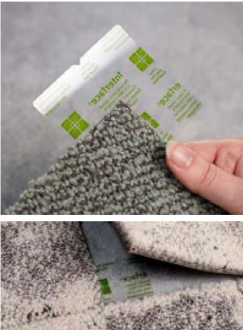
Figure 68: Inspired by the gecko's ability to seemingly "stick" to surfaces, TacTiles® from Interface is a glue-free carpet installation that connect carpet tiles to each other and to the subfloor. Removal and replacement of tiles is quick and easy, whether for the replacement of a single damaged tile or the overhauling of the whole office. The subfloor remains clean and the carpet tiles have no glue residue on them, being ready for reuse.
